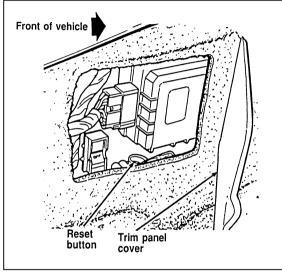
The fuel pump shut-off switch
